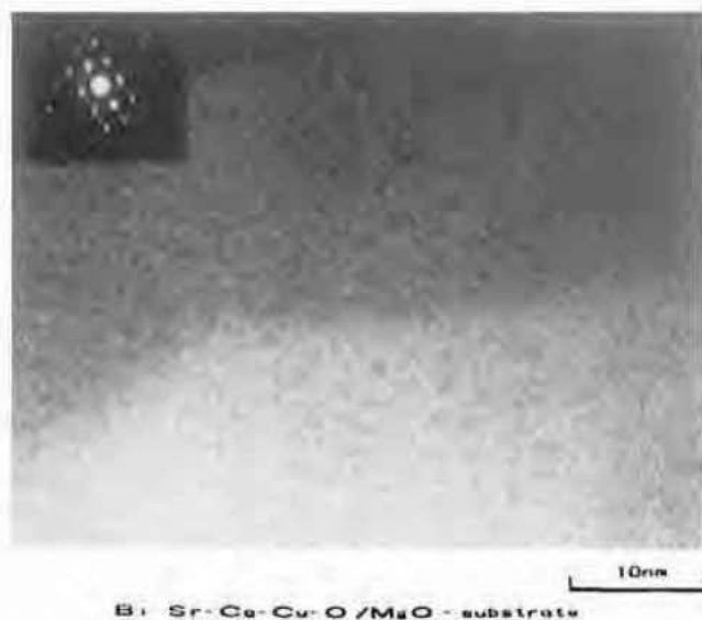
Figure 5.108: TEM image of the sputtered Bi-Sr-Ca-Cu-O thin films of 2-2-1-2 structure.
