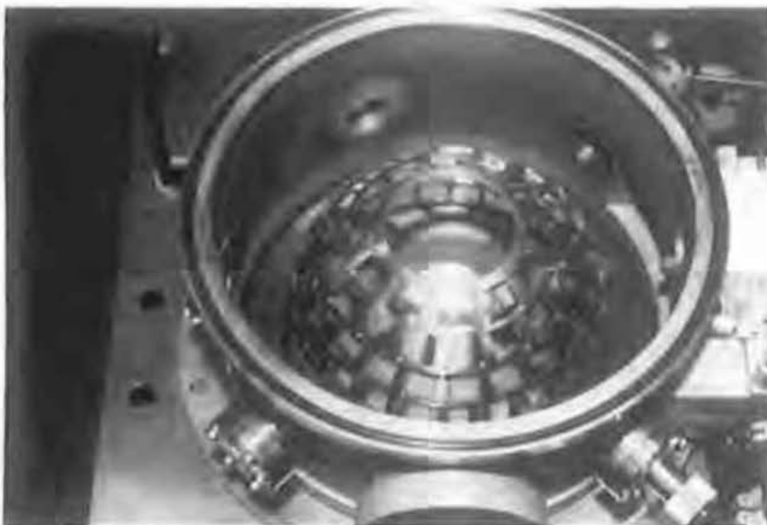
Figure 5.14: Photograph of the sputtering chamber of the hemispherical system with ZnO target.
