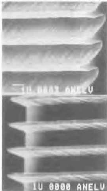
Figure 6.11 Etching structures \text{SiO}_2 on Si prepared by ECR ion beam etching system (9).
